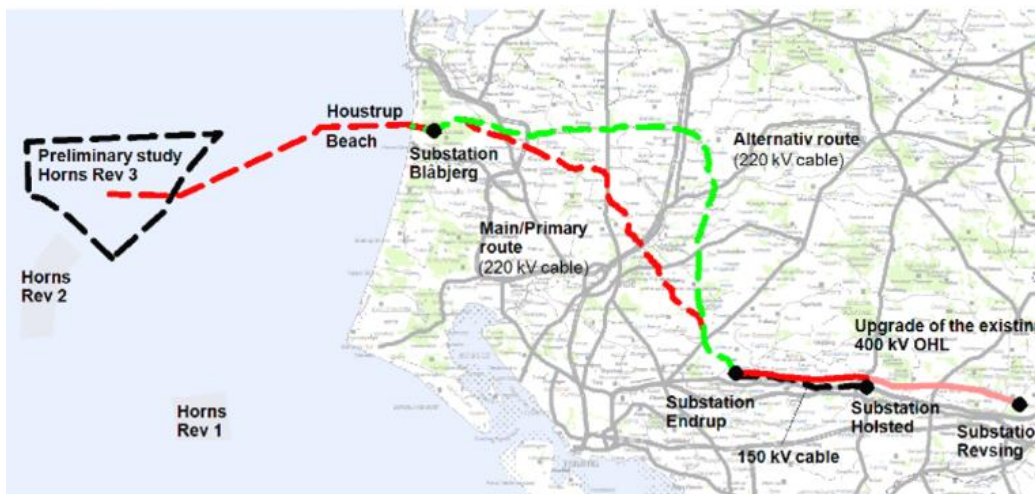
Off- and onshore power cable routing
